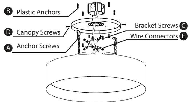
Step 3. Remove Plastic Pin, drill 6 (8mm) holes on the ceiling according the Mounting Bracket. (4 for the Bracket, 2 for safety Bracket Screws). Insert the expansion bolts in the holes. (Use 2 pcs M4x25mm screws to secure the Mounting Bracket with the J-Box), See Fig. 2
