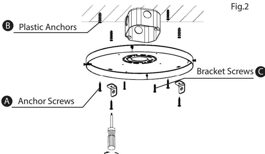
Step 4. Use 6 pcs M4x25 Self-Tapping Screw (2 for Safe Bracket) to fix Mounting Bracket on to the ceiling and connect safety chain between Mounting Bracket and Canopy.
