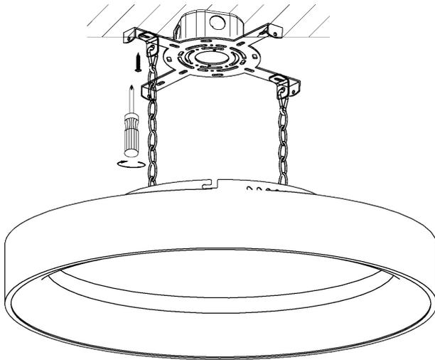
Step 6. Keep the fixture level as possible line up the slots on the bottom fixture mount bracket with the canopy screw. Rotate until both bracket are in place tighten canopy screws to secure it in place.
