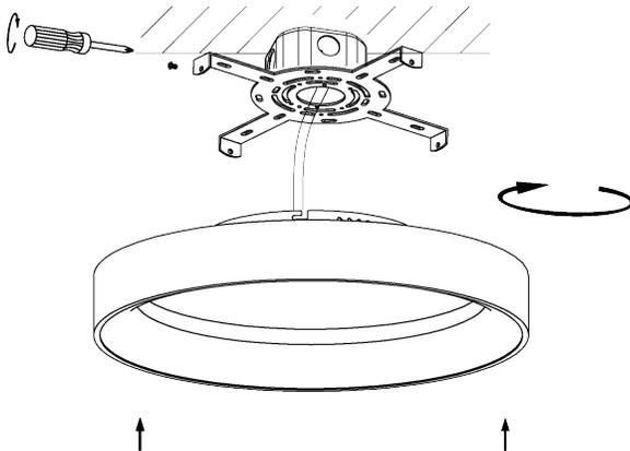
Step 5. Use wire connectors L, N, B, DIM+, DIM - wires. After making the connections place the wires with connectors into the J-Box.
