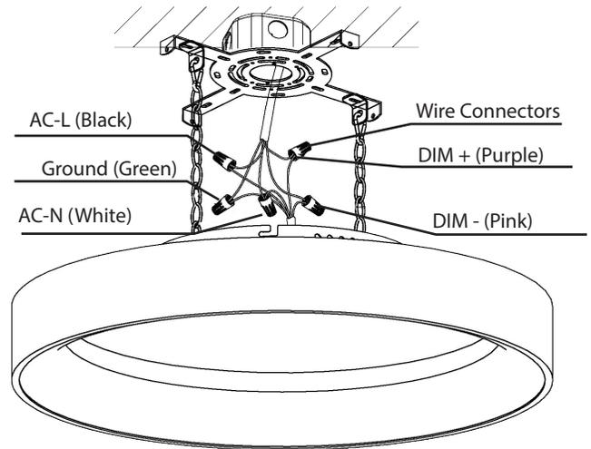
Step 7. Ensure that the fixture is secure. Turn on the power at breaker box or main fuse box to see the fixture is in working order.
