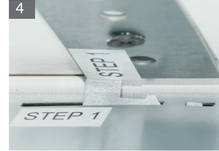
**Step 4:** Align the 2 longer hooks on the metal plate with the longer hole on the luminaire. "STEP 1" is marked on the luminaire. Insert the two longer hooks into the STEP 1 holes. Slightly move the luminaire forward and make sure the hooks are in firmly inserted.
