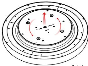
Rotate counterclockwise to remove the surface mount plate
