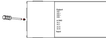
2. Remove round knock-out and connect conduit to wiring box with proper connectors: press the binding post with straight screwdriver, insert the wire and secure. For AC input, connect neutral wire (White) to AC-N, Live wire (Black) to AC-L and Ground wire (Green) to the screw wire logo. For 0-10V dimmer wiring: connect the dimmer(+) wire to the DIM(+) (Purple), connect the dimmer(-) wire to the DIM(-) (Grey).
