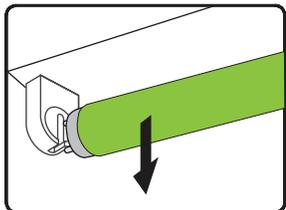
4. Install the LED tube into the lighting fixture.
