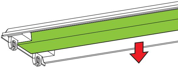
7. Replace the cover over the wiring channel.
