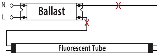
6. Wire Line and Neutral voltage output to opposite ends of the lamp: Hot (L) to one end and Neutral (N) to the other end of the fixture.
