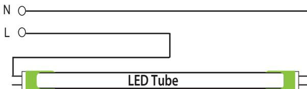
8. Install the LED tube (tube orientation does not matter) and close the Diffuser.
