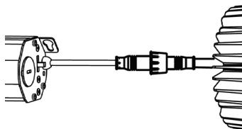
9 Insert the driver through the mud ring trim. Insert the fixture into the mud ring trim and twist to lock into place.
