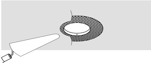
4 Remove the knockout on the junction box and attach Romex connector to junction box.
